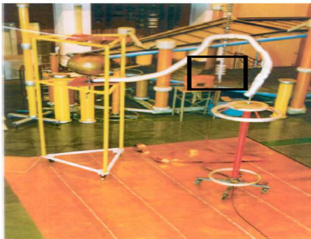
**Fig. 1.** PCI specimen under steep-impulse test.
