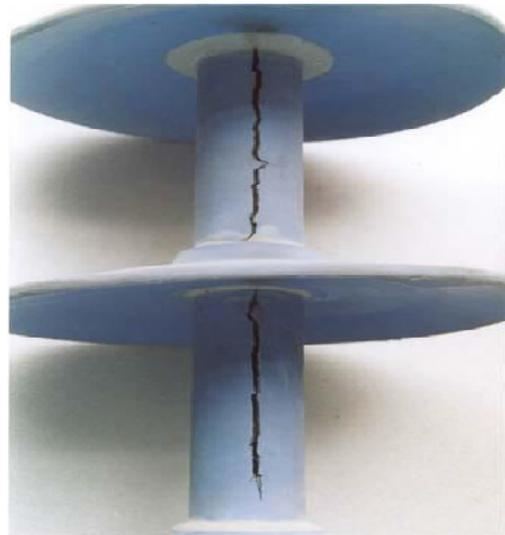
**Fig. 5.** Example of defective (improperly glued to core) housing after 4 kV/ns steep-front impulse test.
