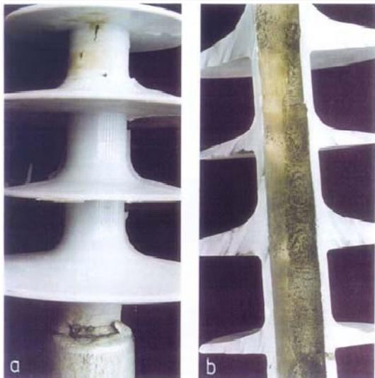
**Fig. 4.** Trace of breakdown on housing and traces of inside discharges along core surface after 4 kV/ns steep-front impulse test.
