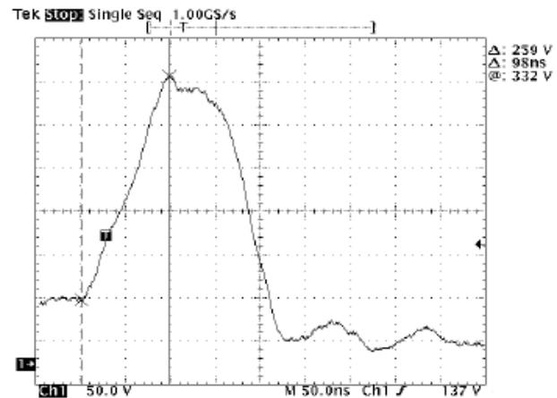
**Fig. 3.** Flashover voltage oscillogram: insulator No. II,  $V = 507$  kV and steepness  $s = 4$  kV/ns.
