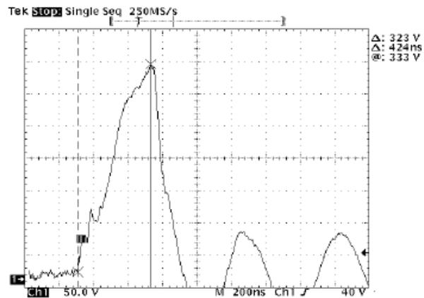
**Fig. 2.** Flashover voltage oscillogram: insulator No. 2.2,  $V = 509$  kV and steepness  $s = 1.2$  kV/ns.
